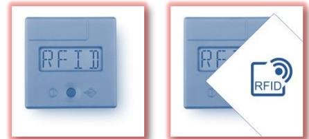
**Note:** Make sure the correct RFID matches the corresponding ImmunoComb/VacciCheck kit. After the **CombCam** is activated with the **RFID card**, multiple teeth of the same kit can be read while skipping the RFID step by pressing the button until **TEST** appears.
